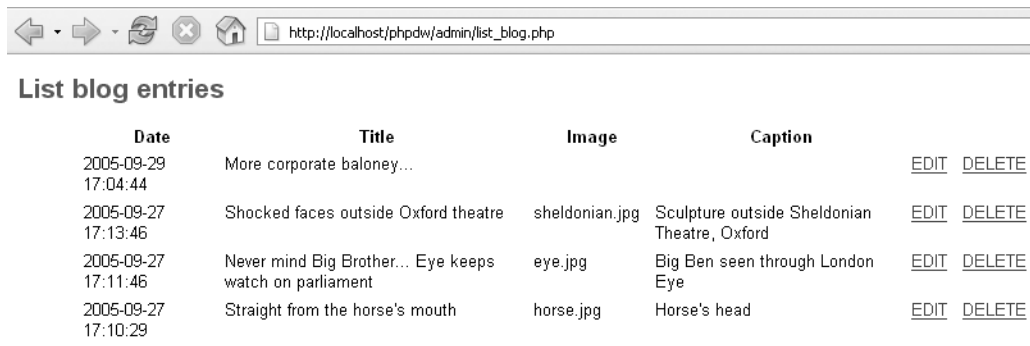
Figure 11-1. The value of the MySQL TIMESTAMP column isn't in a very friendly format.
